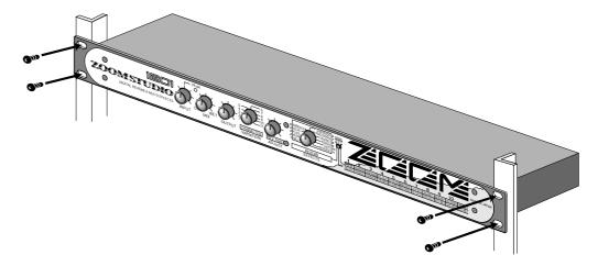
\* Screws for rack mounting are not included with the unit.
