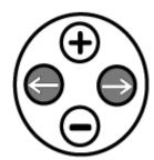
Press either left  $(\leftarrow)$  or right  $(\rightarrow)$  control button to access each specific Function page. You can press and hold either button to scroll quickly.
