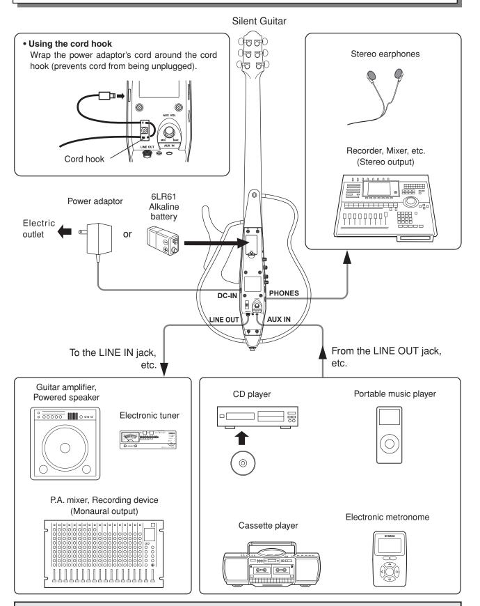
When connecting the instrument to external audio equipment, check the jack size and make sure to use a plug size that corresponds to the jack being used, and properly connect the cable to the jack.
