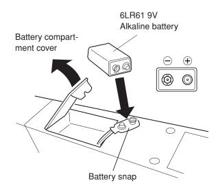
When battery power becomes low, the effect does not operate, the lamp will not light, and noise will be present. Replace the battery with a new alkaline battery as soon as possible.
