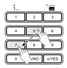
Three-digit voice numbers (i.e. "100" through "169") are entered by first pressing and holding the [1] button until "1" appears in the hundreds position on the display, then press the remaining two digits in sequence.
