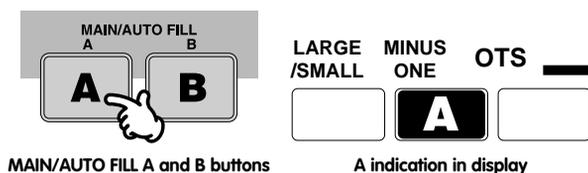
The A or B indication appears in the display, flashing before playback of the pattern and staying lit during playback.
