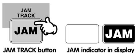
The JAM indicator appears in the display, flashing before playback of the pattern and staying lit during playback.
