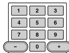
You can either enter the Style number (two digits) directly with the number keys, or step up and down through the Styles by using the +/- keys.
