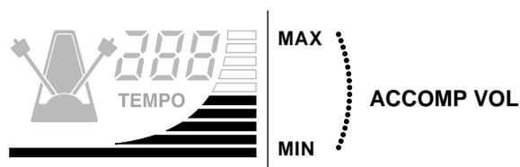
To reset the accompaniment volume to its original default setting, press both ACCOMP VOL buttons simultaneously.
