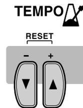
Press TEMPO ▲ to increase the speed and TEMPO ▼ to decrease it; holding down the appropriate button continuously increases/decreases the speed. The tempo value appears in the display. Tempo range is from 40 to 240 bpm (in 1 bpm steps).
