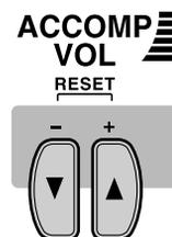
Press ACCOMP VOL ▲ to increase the volume and ACCOMP VOL ▼ to decrease it; holding down the appropriate button continuously increases/decreases the volume. The level is shown in the display.
