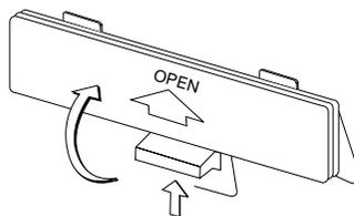
2. Insert six (6) 1.5 V "AA" (R-6, SUM-3) or equivalent batteries into the battery compartment.
