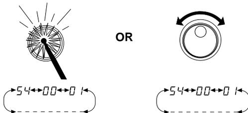
Voice numbers cycle from 00 to 54 to 00 when striking the percussion pad. The ◀ PAD ASSIGN button decreases the voice number and the ▶ PAD ASSIGN button increases the voice number.
