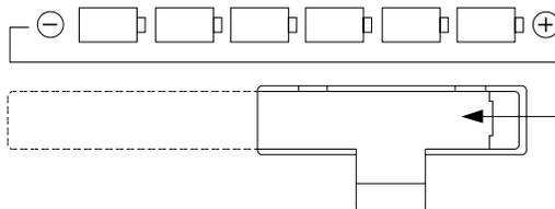
3. Replace the battery compartment cover securely.
