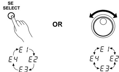
The sound effect set numbers only cycle forward from E1 to E4 when you press the SE SELECT button.
