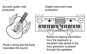
As shown in the illustration above, in an electronic instrument, the sampled note (previously recorded note) stored in the **tone generator section** (electronic circuit) is played based on information received from the keyboard, and output through the speakers.
