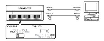
When using a MIDI interface with a Macintosh series computer, connect the RS-422 terminal of the computer (modem or printer terminal) to the MIDI interface, then connect the MIDI OUT terminal on the MIDI interface to the MIDI IN terminal of the CVP-205/203, as shown in the diagram below.
