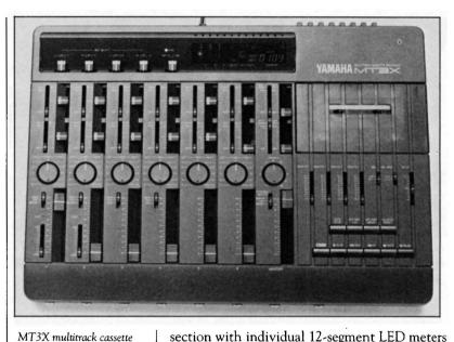
section with individual 12-segment LED meters for each of the four recorder tracks, two 19-segments LED meters in an arced VU-like display for the two Master Stereo busses, a digital electronic tape counter display, and additional status indicators for its unique auto punch-in feature.
