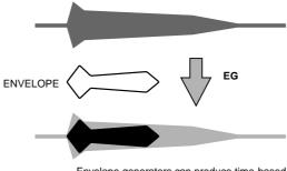
Envelope generators can produce time-based variations in amplitude, filter frecuency or pitch.
