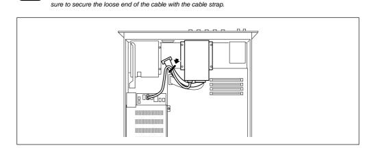
The IDE hard disk is now fully installed. There is no need to remove the disk when installing other devices.
