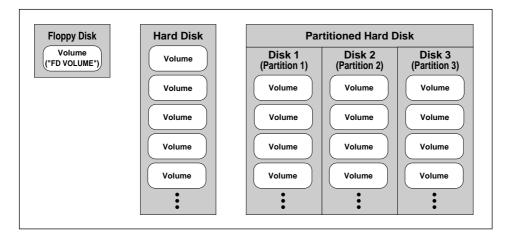
The point to remember here is that each disk volume corresponds exactly to a full set of main-memory data. As the next illustration shows, the A5000/A4000 saves all main-memory data into a single volume. When you reload the volume, you restore the main memory to its exact state at the time of the data save.
