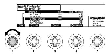
**10.** Rotate Knob 2 to highlight "sine wave," and rotate Knob 4 to set the Receive Channel Assign parameter to "A01" ("01" on the A4000).
