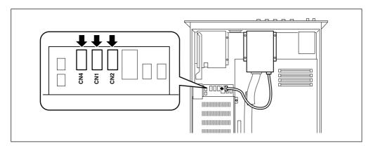
**10.** Install the hard disk and mount panel assembly in the A5000/A4000.
