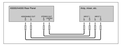
Assignable output using AIEB1 expansion board:
