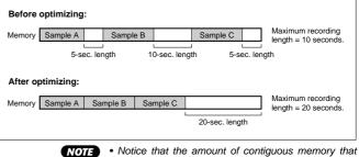
you can obtain by optimizing is indicated on the screen, directly above Knob 4. There is no need to optimize if this value is equivalent to the time value indicated above Knob 2.
