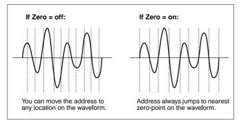
Setting an address on a non-zero point may cause the sample to "click" during playback.
