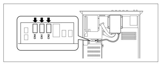
**9** Install the hard disk and mount panel assembly in the A5000/A4000. Refer to page 243 for "Installing an Internal SCSI Hard Disk."
