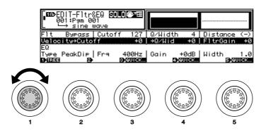
For example, when the EDIT mode FILTER function Filter & EQ page is selected, as shown in the example above, rotating Knob 1 clockwise will move the cursor down line-by-line until the bottom line is reached, then if the Knob is rotated more the next page — Filter Scaling — will be selected.
