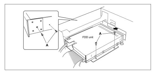
**6.** Turn the FDD unit over, and remove the mount panel from the drive by removing the four gold-colored screws.
