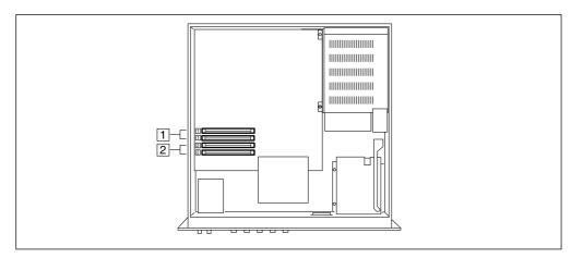
If you are using different SIMM sizes in the two banks, the larger size must be installed into the Bank 1 sockets to ensure that the A5000/A4000 handles the memory correctly. For example, if you are adding one pair of 32MB SIMMs and one pair of 8MB SIMMs, you must install the 32MB SIMMs into Bank 1. If you already have SIMMs installed in Bank 1 and are now adding a larger pair, you will need to move the original pair into Bank 2 and insert the new pair into Bank 1.
