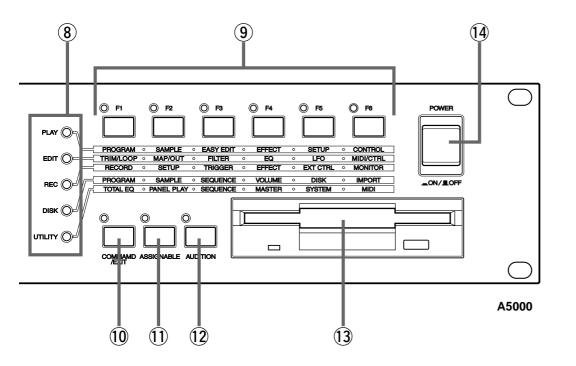
(The A5000/A4000 also uses the button lamps to let you know that it is receiving MIDI data. Each lamp corresponds to a different MIDI data type, and will continue to blink while the A5000/A4000 is receiving MIDI data of that type. (page 85))
