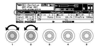
In addition to "New," you can select "New+" to append the recorded data to the end of the currently selected sample, "Replc" to replace a specified existing sample, or "Save" to automatically save the recorded data to disk. See page 153 for details.
