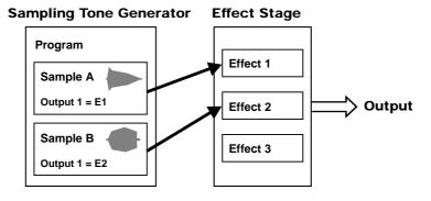
NOTE • The routing of sample output to the effects is carried out via the sample parameters, but the actual effect settings are accessed via the program parameters.
