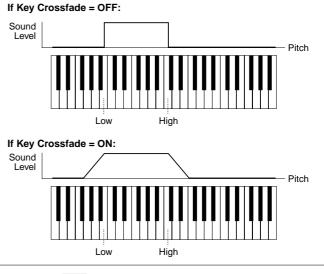
NOTE • The use of key crossfade allows you to blend adjacent samples into one another, so as to avoid dramatic voice changes at the range borders. This is particularly useful when working with samples that map the same type of sound to different ranges on the keyboard (multisampling).
