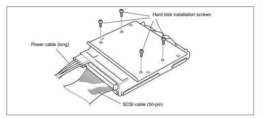
**&** Connect the hard disk SCSI cable (50-pin) to the connector on the A5000/A4000 circuit board.
