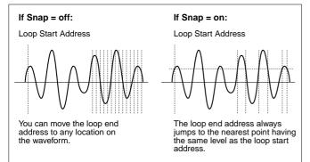
Setting the two loop addresses to different levels on the waveform may cause a "click" sound at the loop point during playback. Forcing the loop start and loop end addresses to the same level will ensure that you avoid this problem.
