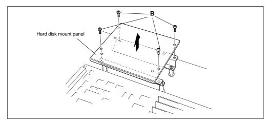
**6.** Attach the hard disk to the hard disk mount panel with the four hard disk installation screws.
