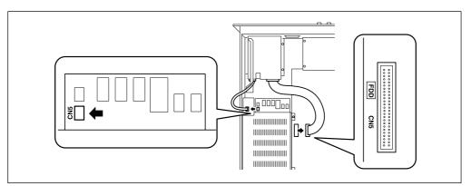
**5.** Remove the four gold-colored screws with which the FDD is attached, and slide the FDD backward (toward the rear panel) to remove it.
