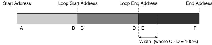
Step 1: Copy waveform piece from start of segment C-D into a buffer. Extract equal piece from the start of E-F, and copy into another buffer. The lengths of these pieces is determined by the Width setting.
