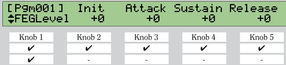
Use this page together with the FEGRate page (☞192) to set up the sample's FEG (filter envelope generator). The FEG determines how the filter's cutoff frequency shifts over time as each note plays out.
