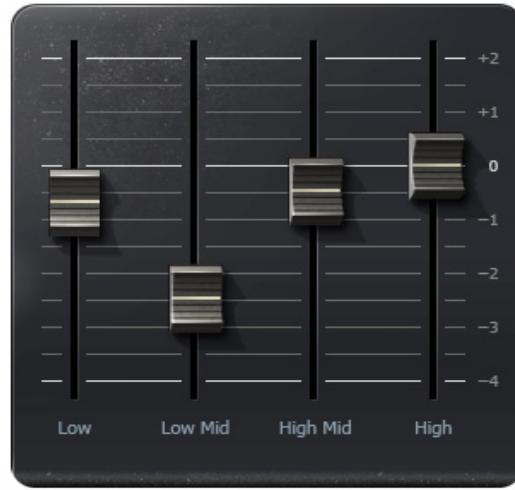
**RANGE FADERS** determine the amount of noise reduction applied to each band.
