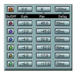
Gain, Pan and Delay Controls
