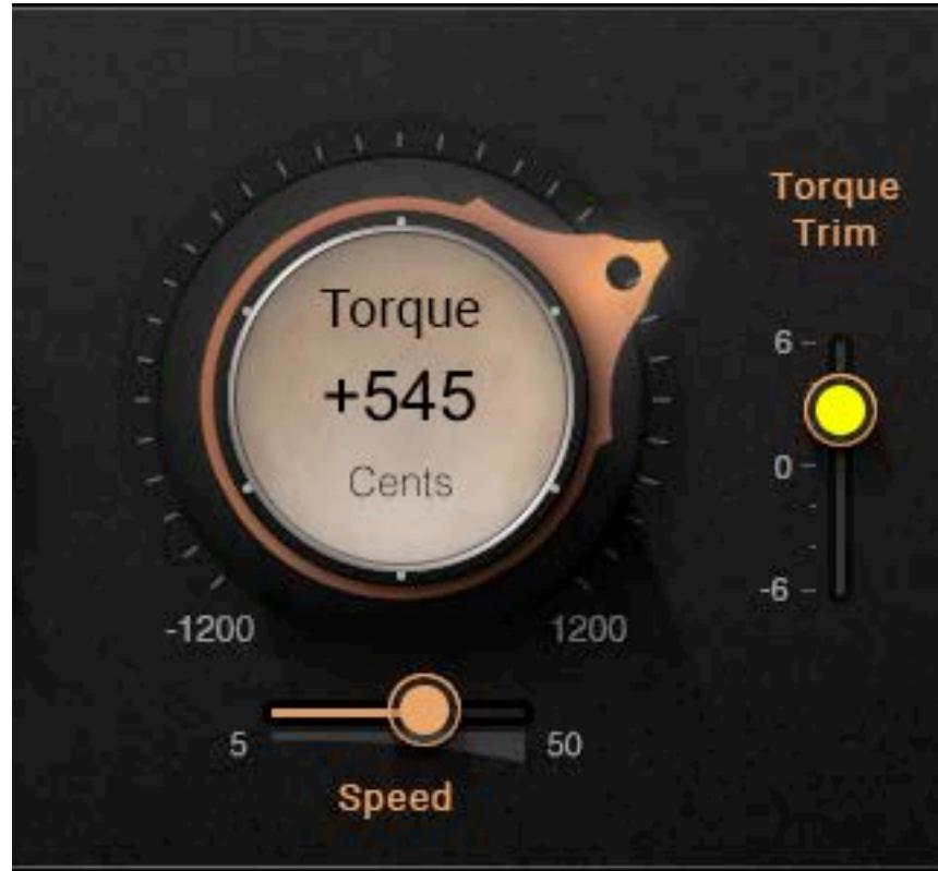
The **Torque Knob** controls the amount of formant shift. This action mostly affects the frequencies around the Focus setting. So if Torque is not correcting tone as expected, re-adjust the Focus setting.
