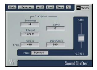
The SoundShifter Pitch is a replica of the Pitch section of the Parametric SoundShifter. Since the Pitch shifting application maintains the duration, this process is adequate for real-time processing as a channel insert. It introduces a fixed amount of pure delay or inherent latency.
