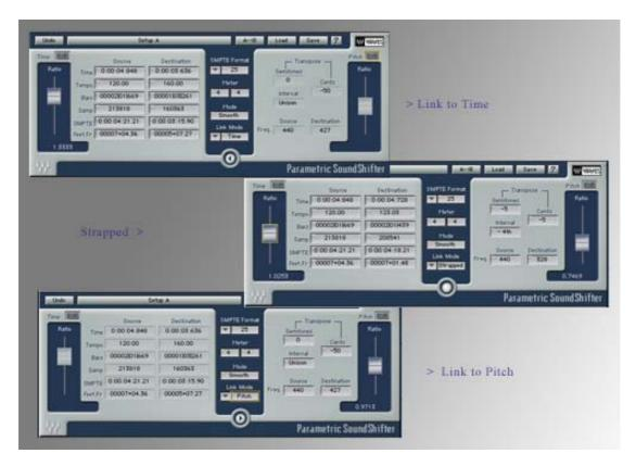
Note that in the Time or Pitch Link modes, the interface will show an arrow pointing to the section that is now dominating the process. The controls of the other section are disabled and therefore appear faded and the Ratio disappears. The disabled section will store whatever settings are there and these settings will get back into action when the link mode is changed.
