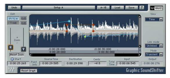
The Graphic SoundShifter takes the very same elements and allows you to program a value change graph across the selection. This is achieved by creating "Points" in the graph that you can drag around to designated timing in the selection at the X axis and to its shift ratio at the Y axis. There are two separate graphs, one for Pitch and one for Time. You can select which one you are editing.
