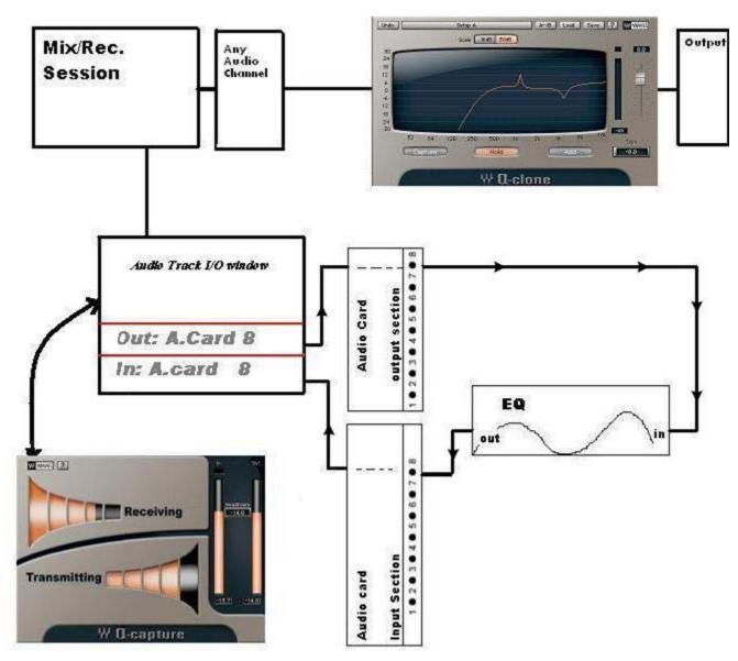
Once the test-signal returns from the device, it is analyzed and loaded into the Q-Clone component as an impulse-response. This happens several times per second so that the EQ-settings of the device are well tracked by the cloned EQ.
