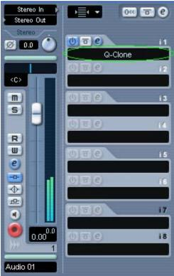
12. Make sure that the I/O on this channel is different than the I/O on the Q-Capture's channel.
