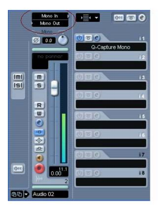
8. Put the Q-Capture in the first Nuendo/Cubase Insert slot. It will be located in the Waves Plug-In list.
