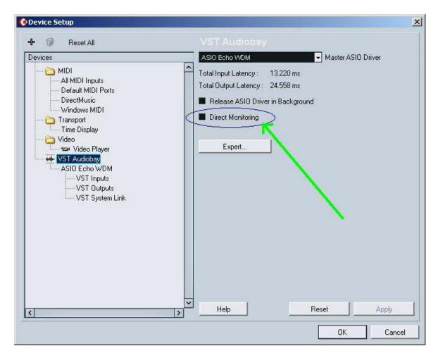
7. Set the I/O of this track to match the insert I/O that you used in steps 1 & 2. The basic I/O setting can be done from the Nuendo/Cubase Menu Bar under Devices>VST Connections (as seen in the following pictures).
