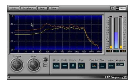
The PAZ frequency analysis is done in bands very similar to those of the ear. The default setting of the **LF resolution** control is 40Hz, which gives 52 bands, and most closely approximates the constant-Q critical frequency bands of the ear. The result is a good correlation between what we heard and what we see in the PAZ frequency analyzer.
