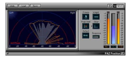
Out-of-phase signals are shown between 45 and 90 degrees on each side. In the area beyond 60 degrees on each side have a red color in the background to indicate that signals in this range might be disturbing to the ears.
