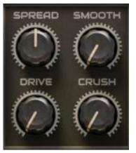
**Spread** – Determines the cut-off offset amount between the left and right channels. Values: -50% to +50% - Default: 0%.
