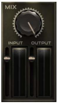
**MIX** – Controls the balance between the "dry" unprocessed source signal and the "wet" processed signal.
