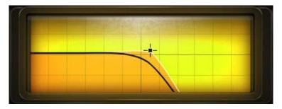
The Graphic Window provides a visual representation of effect MetaFilter applies to the audio signal. The display can be interactively used to simultaneously control the FEQ/RES or **DELAY/FDBK** settings.
