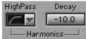
**Highpass filter toggle** - removes low frequencies from the generated harmonics. First position is a 24dB/oct filter at 16Hz (basically to remove DC and very low frequency components); second position is a 12dB/oct filter at the selected Frequency on the graph; third position is a 24dB/oct filter at the selected Frequency on the graph. Default is 12dB/oct.
