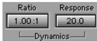
**Ratio** - varies the compression of the generated harmonics. This is an upward compressor, so as the ratio is increased, the level of the harmonics also increase, but with lessened dynamic range. For increased ratios, you will probably need to reduce the Harmonics level fader. The ratio 1:1 has no compression, so the harmonics have exactly the same dynamic character as the Original Bass.
