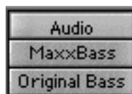
**Monitor button** - selects between Audio (the normal mixed output), Harmonics (the signal created by MaxxBass), and Original Bass.
