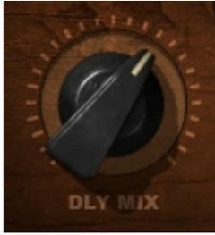
**DLY MIX** controls the audible delay level.
