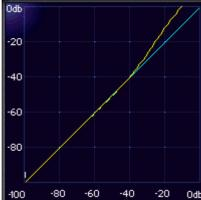
An upward expander from the C1, with a ratio of 0.75:1, Threshold at -35. Equivalent LINMB setting would be a Range of +10 or so, quite a bit more than you'd probably ever need. Shown only for clear example.
