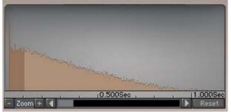
The IR graph shows dB level on the vertical axis and time on the horizontal axis. The range of the IR display is from 0dB at the top to –90dB at the bottom.
