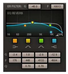
H-Reverb's EQ controls are located near the EQ graph on the left-hand side of the expanded GUI. These include special shelf filters that cut down to -80 dB, effectively behaving like a cut filter. Such a shelf is there for filtering the early reflections, while the reverb tail can be filtered using high and low shelves as well as two bell filters.
