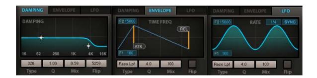
**Damping Mode** is classic and is similar to what's available in many other reverbs. The graph shows the frequency response on the X axis and the reverb time ratio on the Y axis. The damping ratio relates to the reverb time, so if you have a reverb time of 4 seconds and you set the low damping to 400 Hz with a ratio of 1.5, the reverb's mids and highs will decay in four seconds, while the low frequencies of 400 Hz and below will continue two more seconds, taking six seconds to decay fully.
