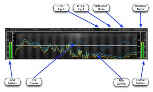
**GRAPHIC DISPLAY / ANALYZER** shows the EQ curve, RTA1 and RTA2 input RMS frequency responses and the Difference between them.
