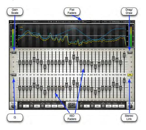
**SCALE** controls the maximum range of GEQ faders. The scale indicators next to the band faders update according to the selected scale. *For example, if the 6 dB scale is selected and 25 Hz is set to +5 dB, changing the scale to 12 dB increases the boost at 25 Hz to +10 dB.* Range: 6, 12, 18 dB
