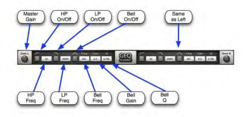
**HP** activates the high pass filter. Range: On, Off
