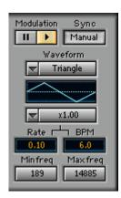
A new control labeled "Sync" has been added at the right-top of the modulation section and it has two modes: Auto and Manual.
