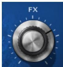
**FX** controls the track's FX send gain.
