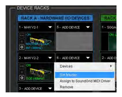
Now you know how to assign I/O devices and designate a device as the clock master. Click on the **Gear** symbol in the device slot to open the DMI Waves Control Panel in order to set up clock details.
