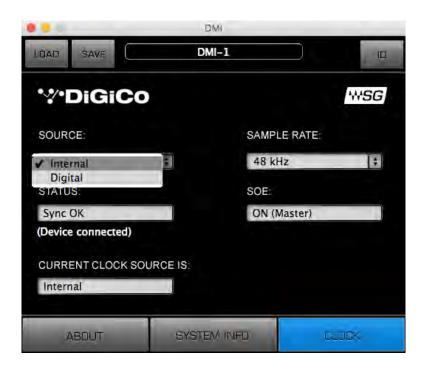
**SAMPLE RATE** sets the sample rate when Clock Source is set to Internal.
