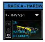
Click on the FW button to launch the Reflasher. This will initiate a scan of the hardware and then offer options. Do not disconnect device or turn off computer until you see "Done."
