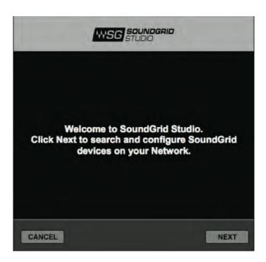
If the Wizard cannot locate the requested SoundGrid network devices, this may mean that the devices might be off or are not connected properly. In such a case the Wizard will allow you to rescan the network or work as a Driver node slaved to another system. For more information please refer the SoundGrid Studio User Guide.
