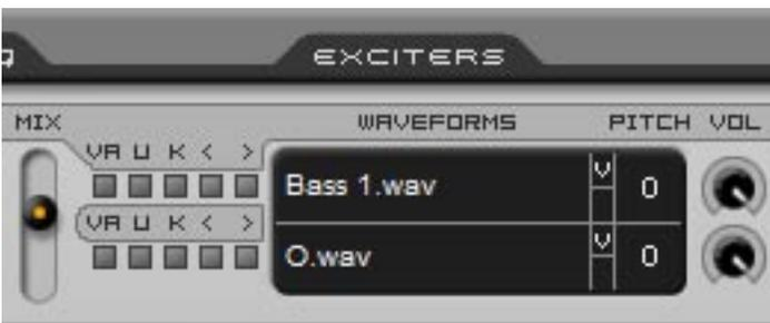
Exciters are what you use to get the delay oscillator moving. As mentioned above, these can be either samples or VA oscillators. The output of both exciters are merged, and that signal is what is sent along to the delays.
