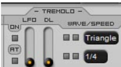
This is an LFO for your volume and, for the most part, it works the same as the other LFOs in M-theory. However, it does have an extra feature of its own. The “**AT**” button lets you use aftertouch to modulate both the rate and depth of the tremolo. The tremolo also has a delay slider, like the pitch LFO has, which lets you adjust how long it takes for the effect to come in.
