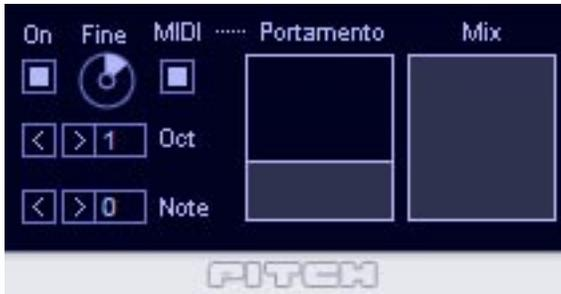
The pitch shifter can be used without the sequencer, and instead can either be set to a fixed increase/decrease, or can be controlled via MIDI input. Note that when the pitch shifter is active but no pitch shifting is set, you will likely still hear a bit of a delay effect.
