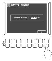
Press the button corresponding to the  $\land$  or  $\lor$  button on the display to change the value.
