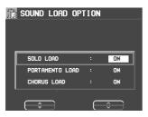
2. Use the ▲ and ▼ buttons to select an item. Use the ∧ and ∨ button to set the filter to ON or OFF.
