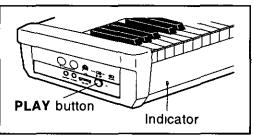
The indicator lamp at the left on the front of the piano lights up when power is on
