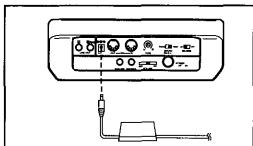
Connect the connecting plug of the AC adaptor (supplied) to the DC IN terminal of the instrument, and the power-supply plug to a wall outlet
