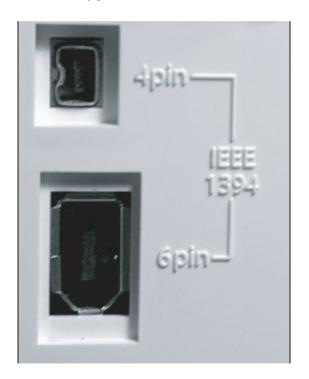
FireOne is supplied with a 2 m (6-foot) cable. If you wish to use a longer cable, the length should not be more than 3 m (9 feet) and the cable should be the best possible quality available to avoid data loss, which results in audio dropouts.
