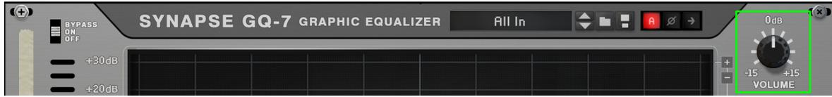
The volume knob adjusts the output level of the GQ-7. By default it is set to 0 dB, neither boosting nor attenuating the output signal. The range of the output volume knob is  $\pm 15$  dB.
