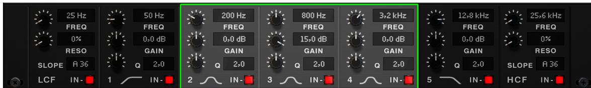
The bell EQ features 3 parameters - frequency, gain and Q. Frequency and Gain can be changed either from the interactive display, or via the corresponding knobs on the bottom panel.
