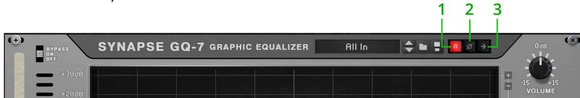
**1) Auto Gain:** Enabling the Auto Gain Compensation (AGC) button automatically compensates for increase or loss of gain caused by the EQ action. Since a louder mix typically sounds better, it is a common mistake to boost too much. Likewise, cutting frequencies may sound worse as the mix becomes softer, even in situations where this is an improvement. The AGC option can substantially speed up the work flow, by compensating for the volume difference after EQ'ing.
