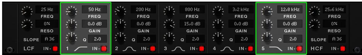
The low shelf filter is primarily designed to boost or attenuate bass frequencies, although it can be used across the entire spectrum. The low shelf EQ features frequency, Q and gain parameters, just like the bell-shaped EQ.
