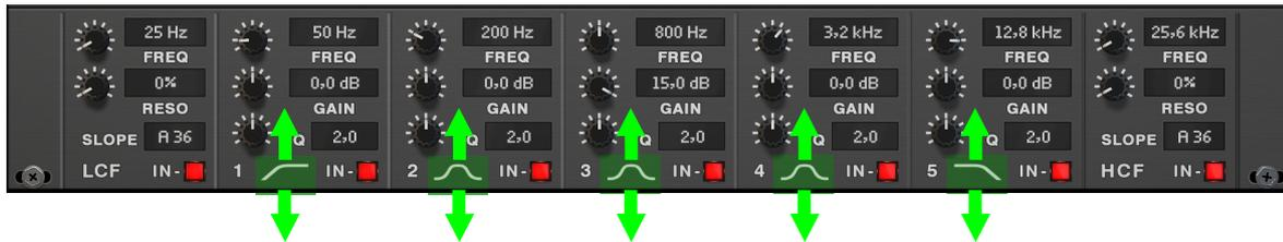
By default, the first and last band are set to low- and high shelf filters, respectively, while bands 2, 3 and 4 are set to a bell filter.
