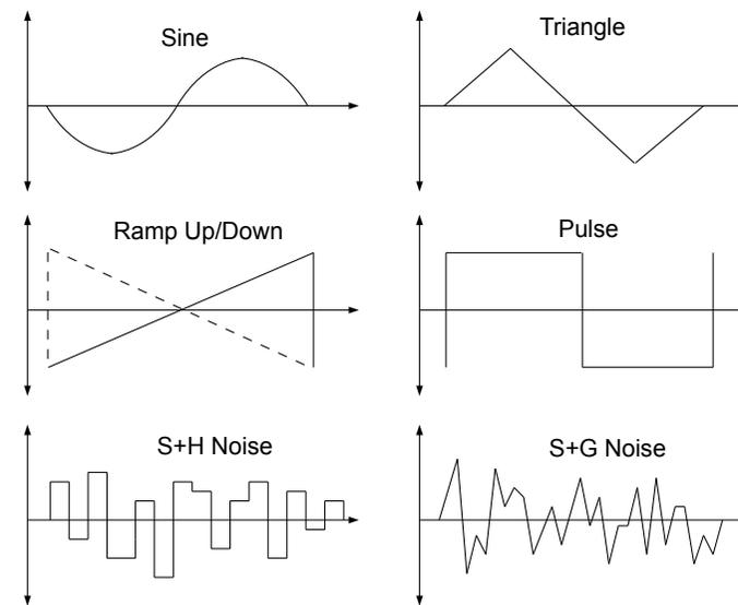
Figure 4.10: LFO waveforms.
