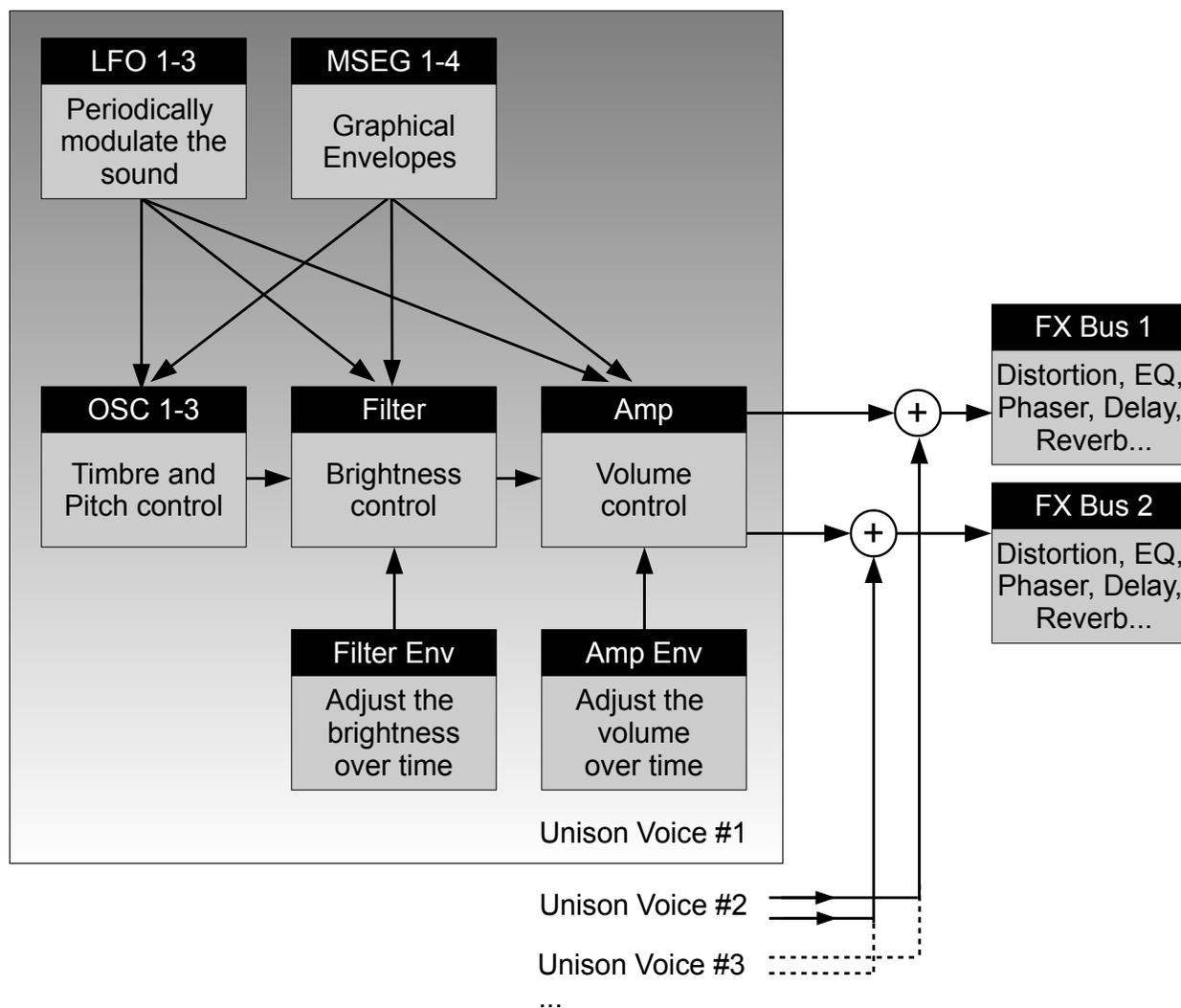
Figure 4.1: Structure of a Dune 2 patch.
