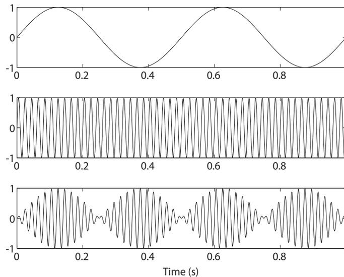
Figure 4.5: Ring modulation of two sine waves.
