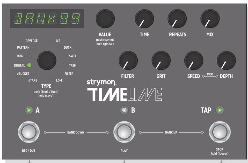
**SPEED:** Controls the speed of the delay modulation LFO
