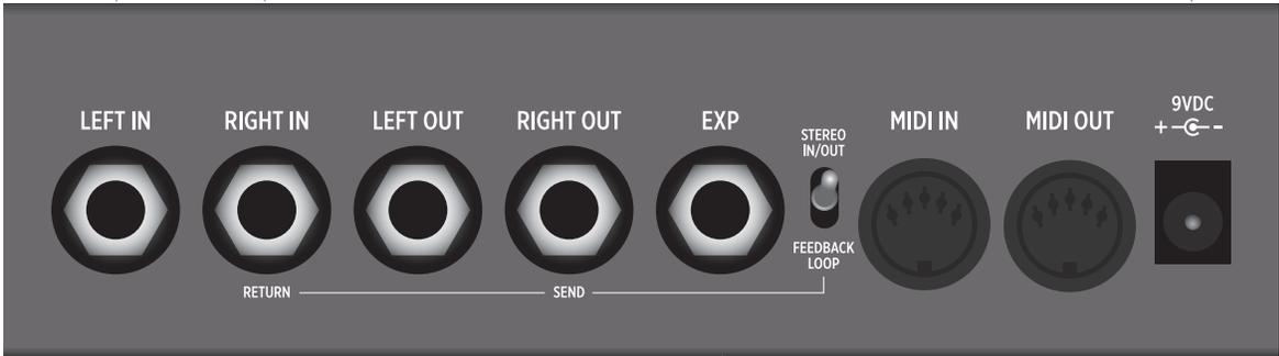
**OUTPUTS:** Use **LEFT** output for mono. **RIGHT OUT** is used as an effect send if the feedback loop is selected.
