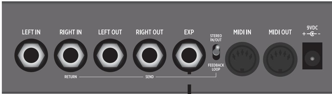
Connect an **external TAP switch** to tap tempo remotely. Use a standard TRS cable to connect the external switch. Set the EXP MD global setting to TAP to use external tap.
