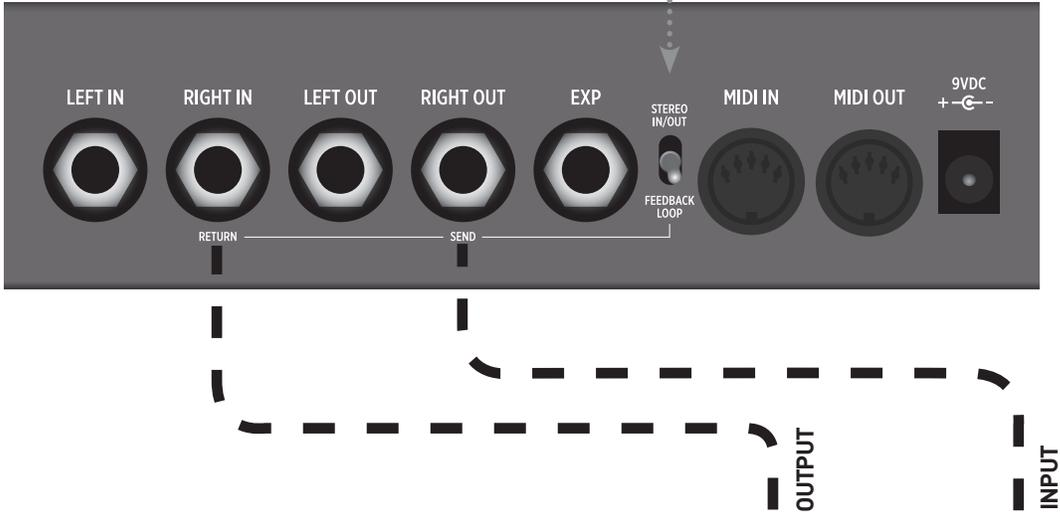
Connect an **external effect** to the feedback loop. Any external effect can be used. Feel free to experiment with the different sounds that can be achieved. All of the delay repeats will be processed through the external effect.
