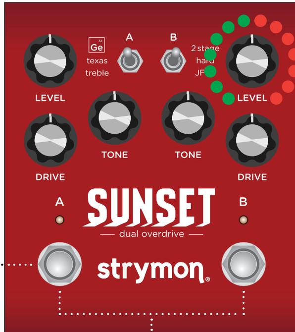
2 Turn the LEVEL knob on the B side to set the EXP jack mode.
