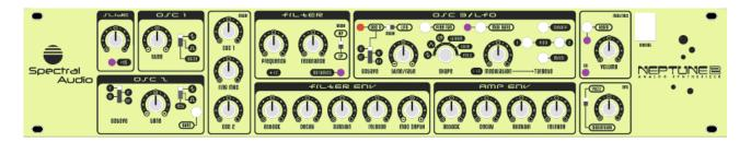
The basic principle of the Neptune II corresponds to classic subtractive analog synthesis which incorporates interconnection between a VCO, VCF, VCA, envelope generators and LFO.
