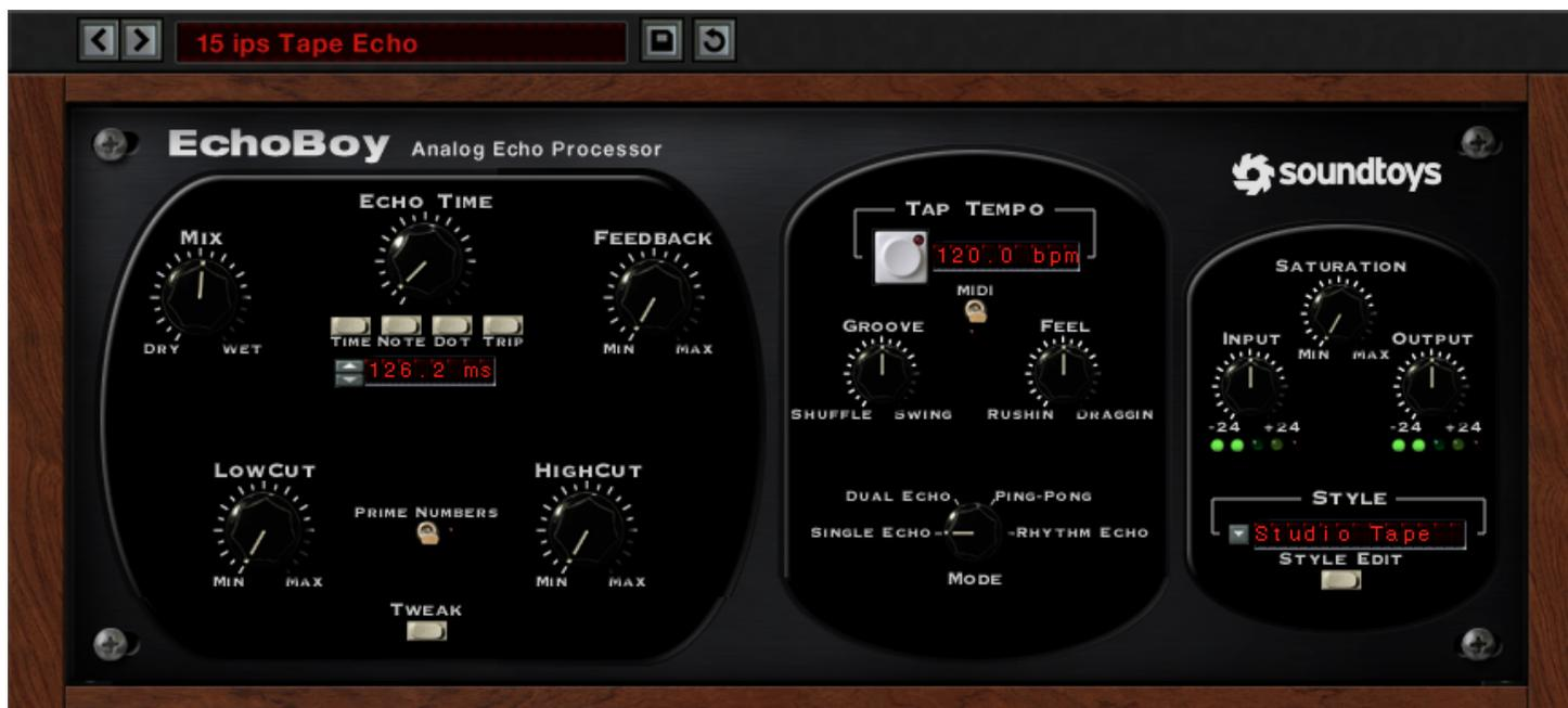
Figure 2: EchoBoy Main Control Panel (Single Echo Mode)
