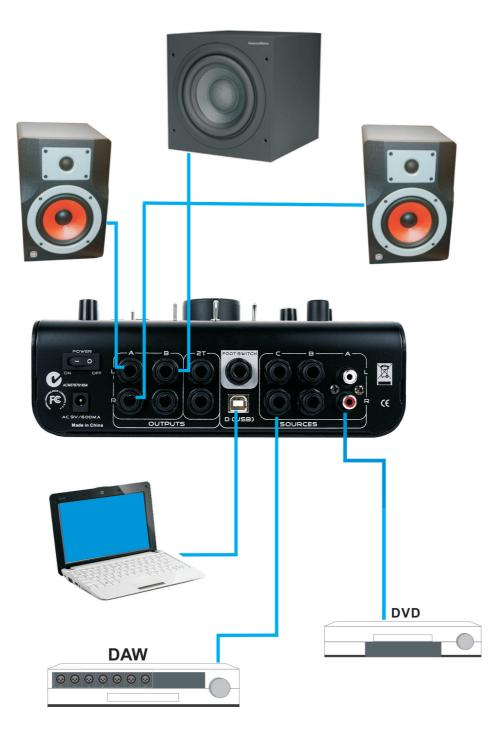
When connecting PASSIVE speakers, you must first connect the output of the ACTIVE-1 to your amplifier and then connect the amplifier to the speakers.
