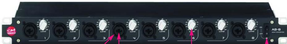
4.4 Front Panel Combo line input 4.3 Combo input XLR
