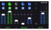
On-screen label text describes the SINGLE TAP commands of the bottom three buttons
