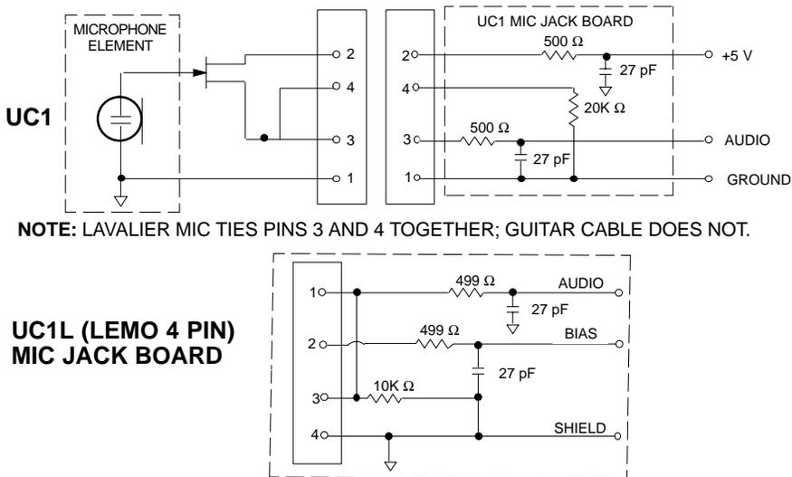
**NOTE:** LAVALIER MIC TIES PINS 3 AND 4 TOGETHER; GUITAR CABLE DOES NOT.
