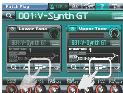
3. Use the section tabs at the bottom of the screen to select a section such as OSC or COSM, and use the detail tabs at the left to select detailed settings within that section.
