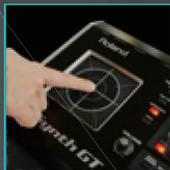
You can apply a variety of effects by touching the Time Trip pad while you hold down keys on the keyboard.
