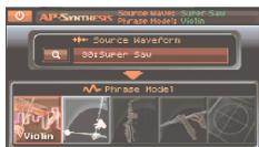
In AP-Synthesis, a "dynamic model" that's distinctive of actually existing acoustic instruments is applied to synthesizer sounds, allowing the "expression" and "movement" characteristic of those instruments to be portrayed, rather than simply reproducing the sound.
