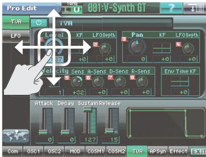
When you touch the <Level> knob, the numerical area will turn blue, and the cursor will move to Level. Continue touching the <Level> knob, and drag your finger up/down or left/right. Dragging your finger up or to the right will increase the value, and dragging it down or to the left will decrease the value.
