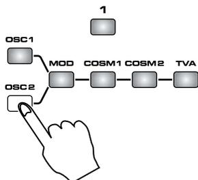
For example if “OSC1” and “OSC2” are both off, there will be no sound-producing section, and no sound will be output.
