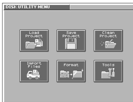
In this mode, you can perform operations related to disks, such as saving data on a disk or loading data from a disk.
