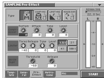
There are three pre-effects: compressor, limiter, and noise suppressor. By using these you can adjust the level of the sound being sampled.
