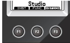
The [F1]–[F3] buttons are called "function buttons." The bottom line of the display indicates the name of the functions performed by [F1]–[F3].
