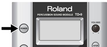
\* The TD-9 is equipped with a protection circuit and requires a brief interval (a few seconds) after powering before it will operate normally.
