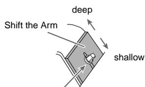
Loosen the bolt with the included tuning key. After adjusting, tighten the bolt.
