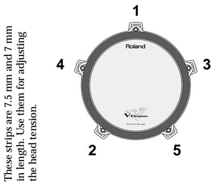
1. Use the included tuning key to tighten the tuning bolts.
