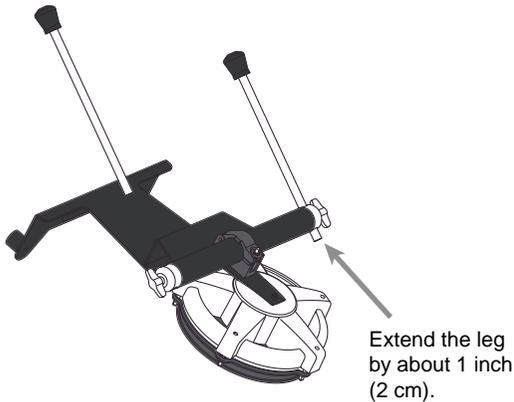
8. Tighten the T-bolts to secure the legs to the stand.
