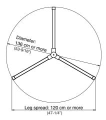
Before use, adjust the speaker stand to a height of 140 cm (55-1/8") or less and a leg spread of 120 cm (47-1/4") or more, as shown in the figure below.
