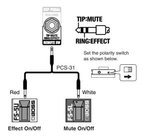
\* If using a FS-6 switch, set the MODE and POLARITY switches as shown below.
