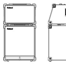
Adjust the horizontal position of the top cabinet so that the corner protectors are properly engaged and locked at all four corners between the top and bottom cabinets.
