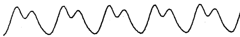
Reverberation wave of an electric Piano 1.5 second after the attack When the reverberations calm down, wave-forms become gentle.
