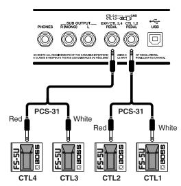
\* If you want to connect foot switches individually, the CTL1 pedal function and CTL3 pedal function settings are used.
