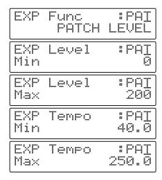
3. After using PARAMETER [ ☐ ] [ ☐ ] to move the cursor to "SYS" or "PAT" in the upper row of the display, you can then rotate the PATCH/VALUE dial to select either the system settings or patch settings as the settings to be used.
