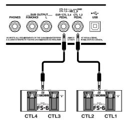
\* When connecting two foot switches with the special connection cable (Roland PCS-31; optional, sold separately), the correspondence between pedal switch and CTL pedal functions is as shown below.
