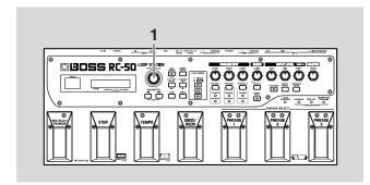
In the Play screen, rotate the PATCH/VALUE dial to switch to a patch.
