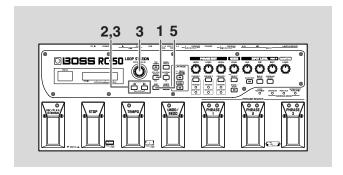
1. Press [CTL/EXP PEDAL] to display the pedal settings screen.
