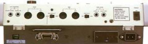
The MIDI-compatible MSQ-700 accepts all MIDI information, including pitch, velocity, MIDI channels, Patch memory changes, Hold function, and Bender operation, and reproduces all the data faithfully.
